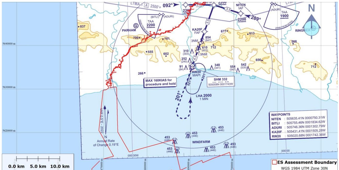
Graphic 2-4 Extract of Required Navigation Performance (RNP) procedure for Runway 20 at Shoreham Airport
